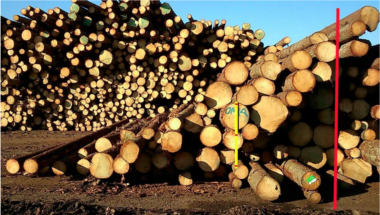
FIGURE 7 DIVIDING THE STACK
