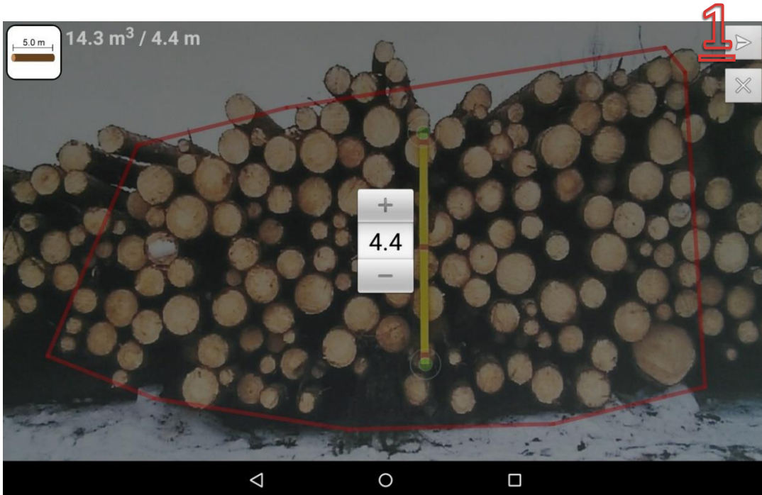
FIGURE 6 INPUTTING THE STACK LENGTH
