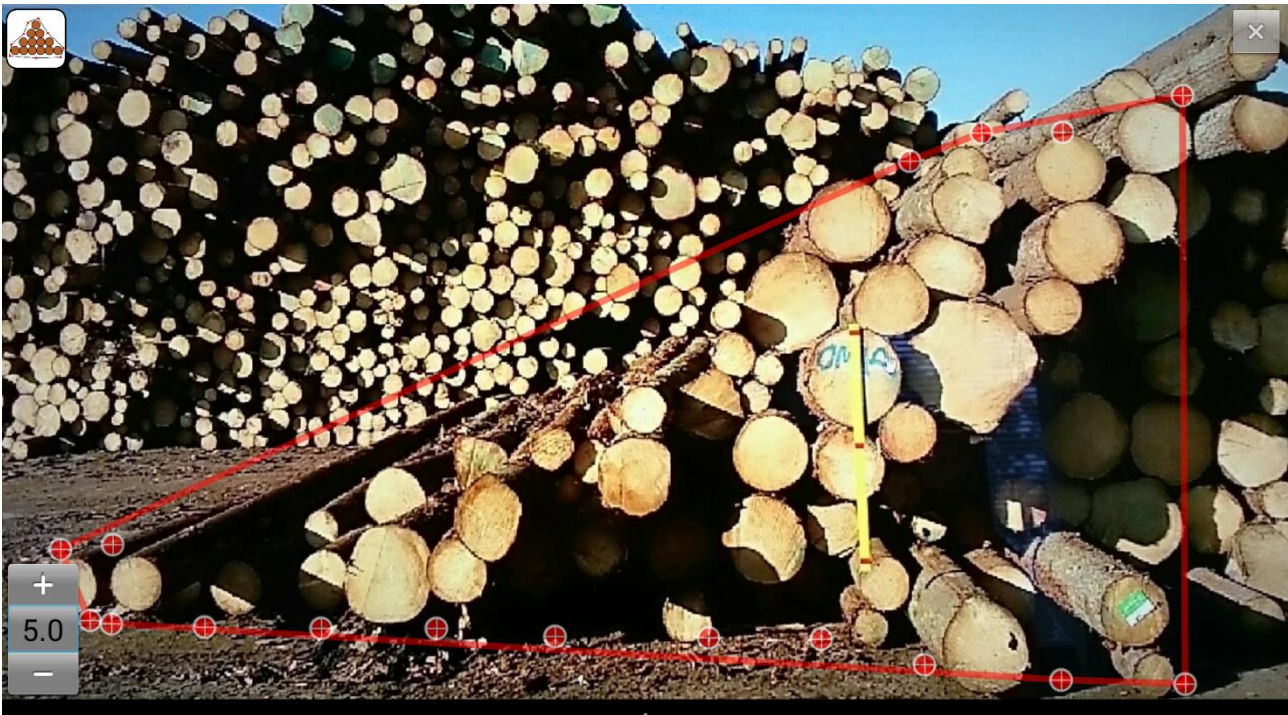
FIGURE 8 EXAMPLE BOUNDARY POINTS FOR A STACK SECTION
